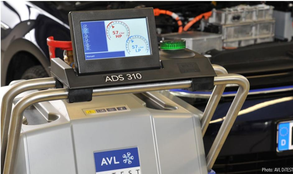
The ADS 310 air conditioning service device makes fast, secure and cost-effective servicing of R744 climate control systems possible.
