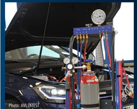
The leak test shows whether the system is airtight.
