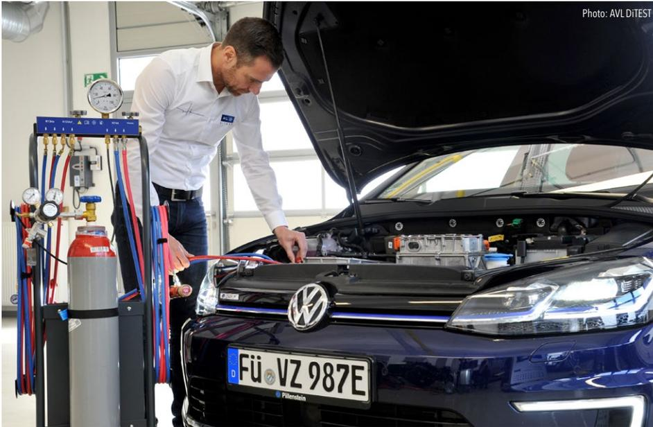
The DPG 1300 from AVL DiTEST can be used on all current climate control systems, regardless of the coolant used.
